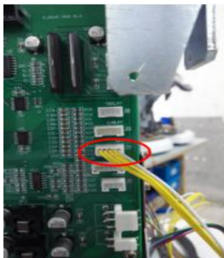
The diagram of the connection between motor driver board and key board
