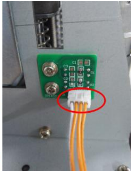
The diagram of the connection between motor driver board and main lift motor limit board
