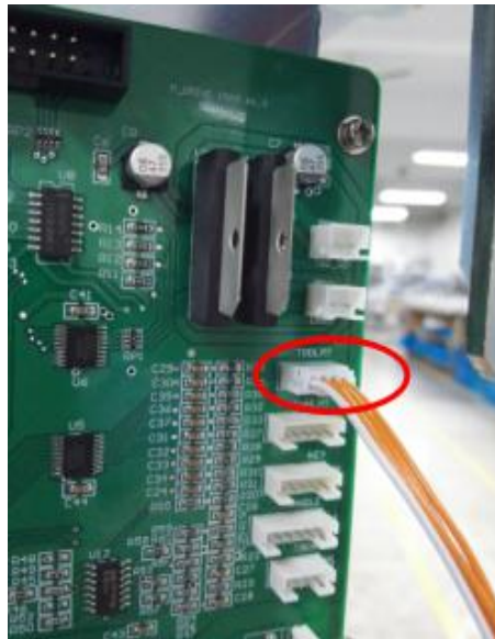
The diagram of the connection between motor driver board and main lift motor limit board
