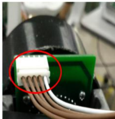
The diagram of the connection between LED driver board and LED light board
