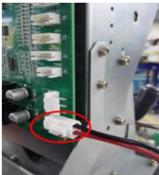
The diagram of the connection between motor driver board and printer board
