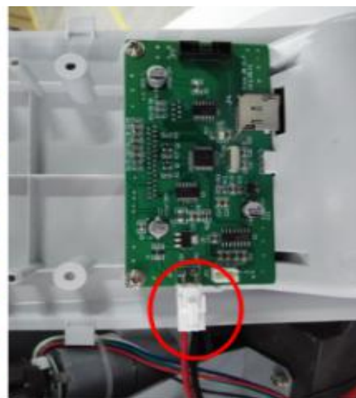
The diagram of the connection between motor driver board and printer board
